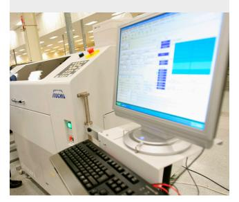
At each screen, the manufacturing cell staff are able to see a real-time display of the status of the jobs running on each machine within their area. To initiate a new job, the operator touches the machine or process that he is running, and a list of jobs in priority order is displayed. Full traceability of labour is provided by the use of RFID (radio frequency identification) tags used by operators to log and log off jobs at the touch screen terminal.
